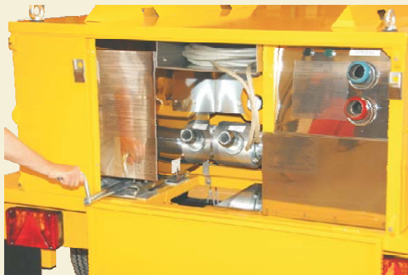
Regulation of cellular concrete flow
